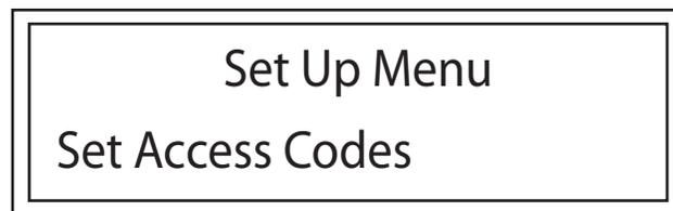
Step 2. Select the Code # you would like to Set using the up or down buttons. Press the Enter button
