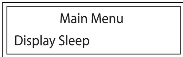
Step 2. Press the Enter button to send the display into sleep mode. No other prompts will be offered. You will simply enter sleep mode by pressing the Enter button.
