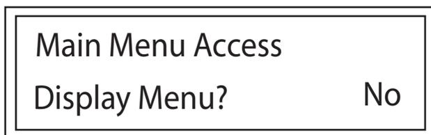
Step 4. Use the up and down buttons to select yes or no and press enter. Yes will allow access to the Display Menu. No will prohibit access to the Display Menu.
