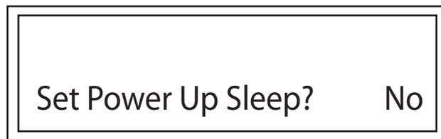
Step 2. Use the up and down buttons to select yes or no. Yes will make the organ enter sleep mode after each powering up. No will make the organ power up normally. When you have selected yes or no press the enter button.
