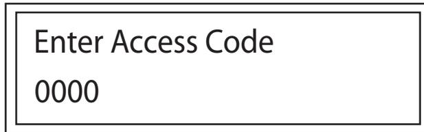
Step 2. Use the Up or Down Buttons to select the first number and press the enter button to advance to the next number in the code. Once the desired Code is input, press the enter button.
