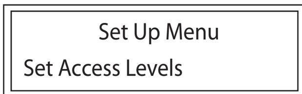
Step 2. Using the directional buttons, scroll through the list of Access Codes until the desired Access Code is displayed. Press the enter button.
