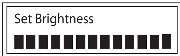
Step 2. Use the Up or Down Buttons to select the desired level of Brightness. Once the desired level of brightness is selected, press the enter button.
